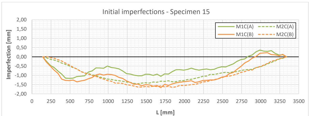
Figure B.17: Initial imperfections of both faces along specimen 15
