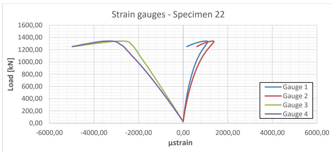
Figure B.32: Measurements of strain gauges on specimen 22
